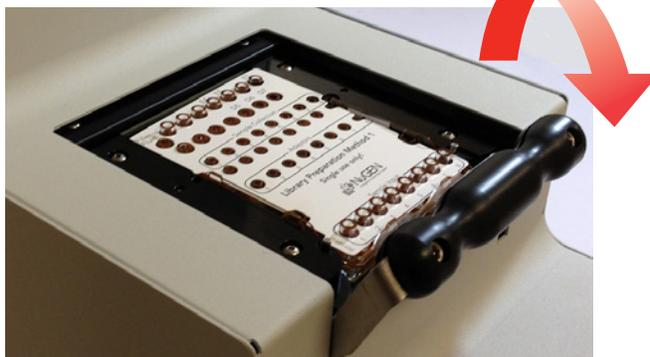
**Note:** Once a run has started, do not move the locking lever as this will result in an unrecoverable interruption of the running protocol. The Mondrian SP+ Workstation will not run with the lever in the up position.
