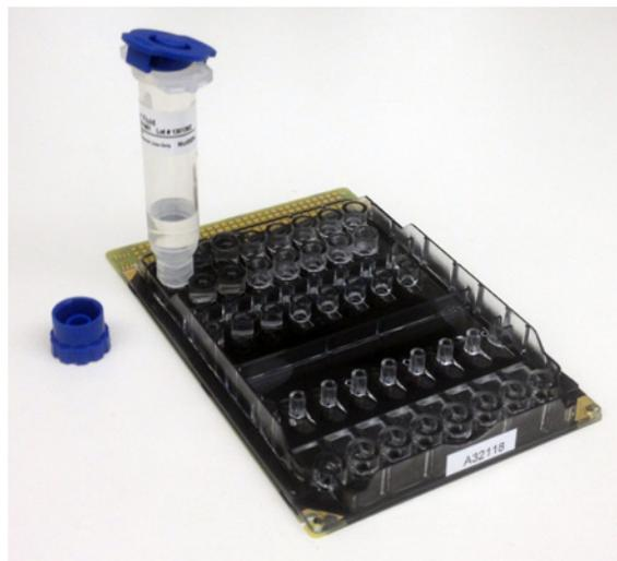
During the cartridge filling process, you will begin to see the filler fluid rising in the sample and reagent ports. You should see filler fluid in all sample and reagent ports by the end of the filling process.
