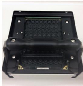
**Figure 4. A close up view of the cartridge alignment marks etched into the deck of the Mondrian SP+ Workstation.** A) no cartridge is inserted. The alignment marks are clearly visible. B) the cartridge is correctly inserted. The points of the guide arrows align with the edge of the cartridge.
