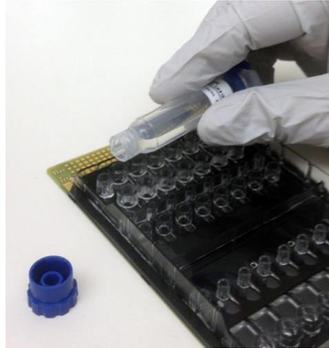
11. Insert the tip of the Filler Fluid tube into the port marked "Filler Fluid" on the SP+ Cartridge while gently twisting the tube in a clockwise direction to seat the tip of the Filler Fluid tube into the cartridge port. Remove the top cover from the Filler Fluid tube, allowing the entire volume of Filler Fluid to flow into the cartridge. This process will take approximately 3–5 minutes.
