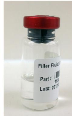
4. Carefully grasp the tab on the red aluminium seal of the SP+ Filler Fluid bottle and pull up and back to break the seal, as shown below.
