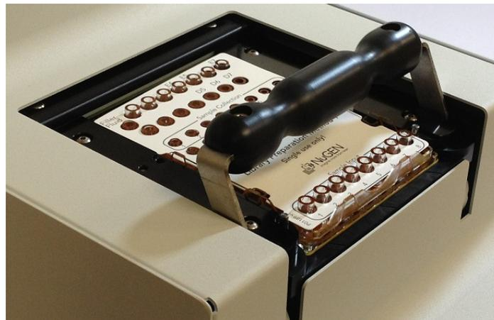
4. Pull the locking lever forward and down as illustrated in Figure 10 to engage the control electronics and lock the cartridge into place.
