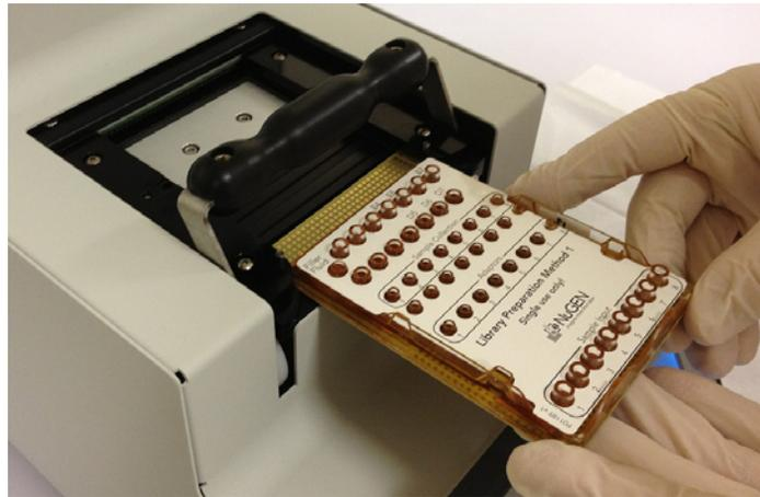
3. Confirm that the cartridge fits snugly into the rear of the deck and that the electrodes are not visible from above (Figure 6). This will ensure that the electrodes will make good contact with the control electronics at the rear of the deck. When the cartridge is properly inserted, three guide arrows etched into the metal surface at the front edge of the deck should be visible with their tips flush with the edge of the cartridge, as illustrated in Figure 8.
