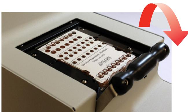
**Note:** Once a run has started, do not raise the lever as this will result in an unrecoverable interruption of the running protocol and an error flag. The Mondrian SP Workstation will not run with the lever in the up position.
