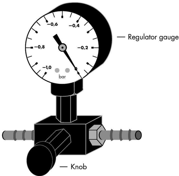
Figure 2. Schematic diagram of the Vacuum Regulator.
