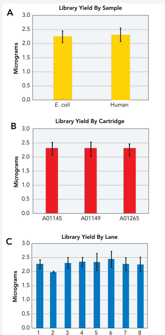
FIGURE 1. Enriched library yields plotted by sample type (A; N=12), cartridge number (B; N=8) and lane number (C; N=3)
